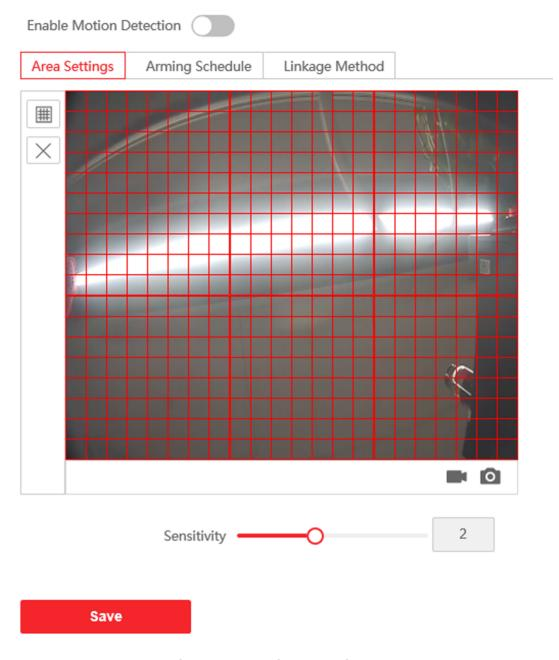
**Figure 5-17 Motion Detection**
