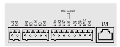
**Figure 2-4 Door Contact Wiring**
