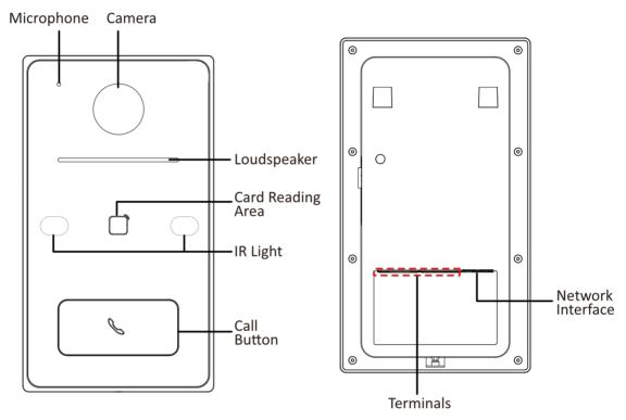
Figure 1-1 Front Panel and Rear Panel
