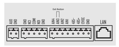
Figure 2-5 Exit Button Wiring
