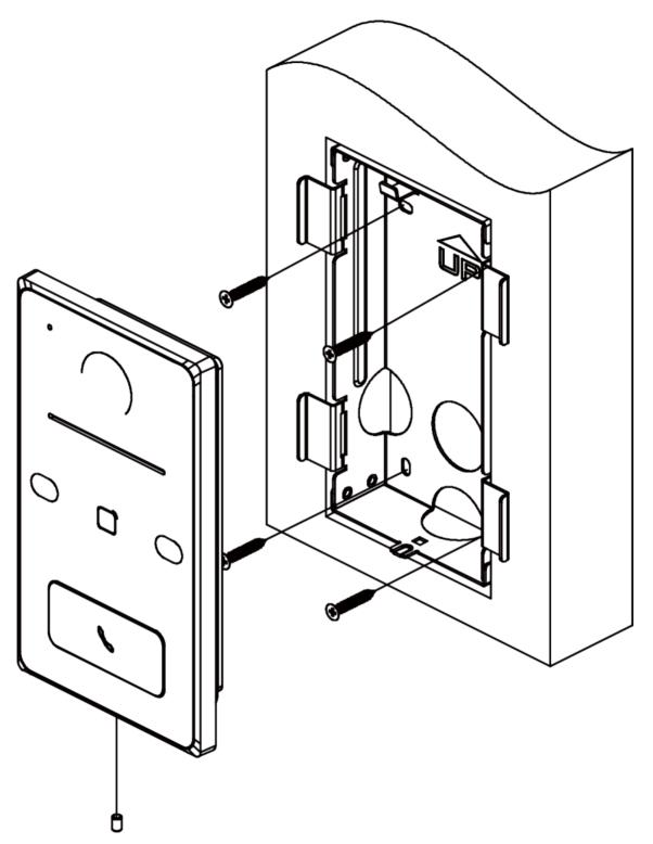
Figure 3-3 Flush Mounting
