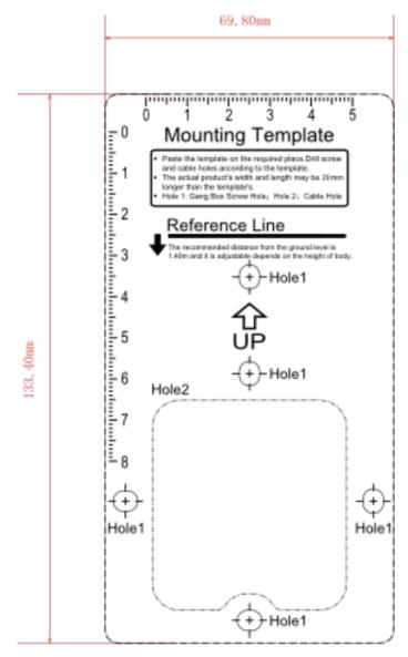
**Figure 3-1 Mounting Template**
